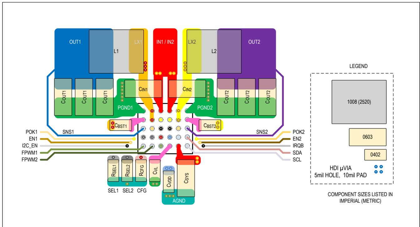
Figure 11. PCB Layout Example
