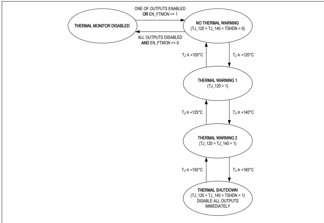
Figure 1. Thermal Warnings and Thermal Shutdown
