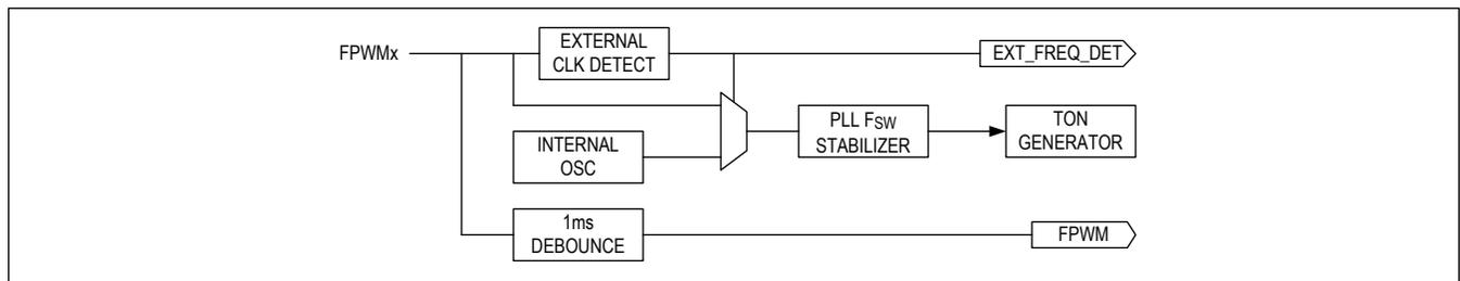
Figure 4. Frequency Tracking
