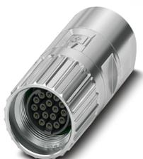
Cable connector, straight, shielded: yes, Screw locking, M17, No. of pos.: 17, type of contact: Socket, Crimp connection, cable diameter range: 5.5 mm ... 9.5 mm, coding:N
