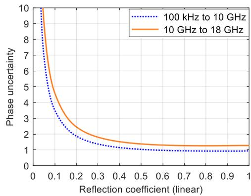
Measured uncertainty of reflection magnitude and reflection phase measurements for the R&S<sup>®</sup>ZNLE<sup>1</sup>; analysis conditions:  $S_{12} = S_{21} = 0$ , calibrated power -10 dBm, measured power -10 dBm
