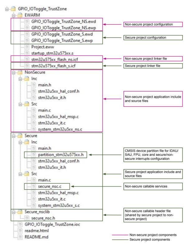
The STM32CubeU5 firmware package provides default memory partitioning in the *partition\_<device>.h* files available under:
