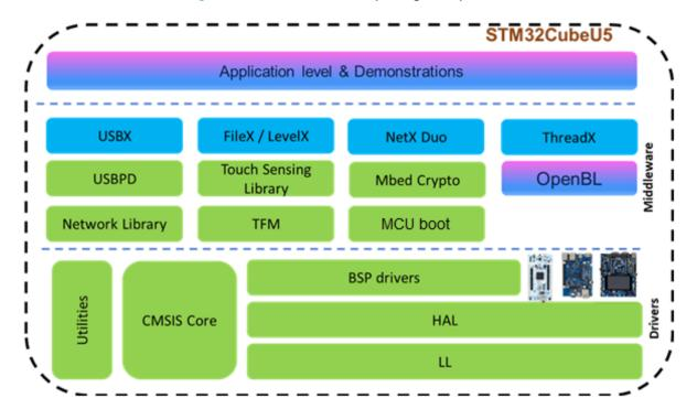
Figure 1. STM32CubeU5 MCU package components
