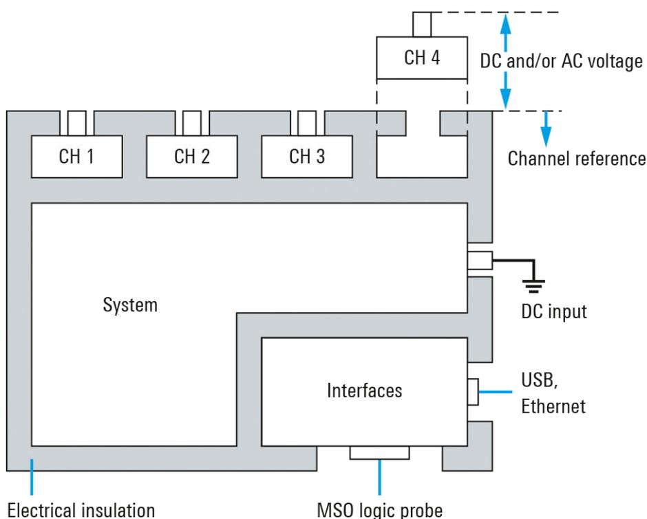
**Figure 2-1: Isolation scheme of the R&S RTH**
