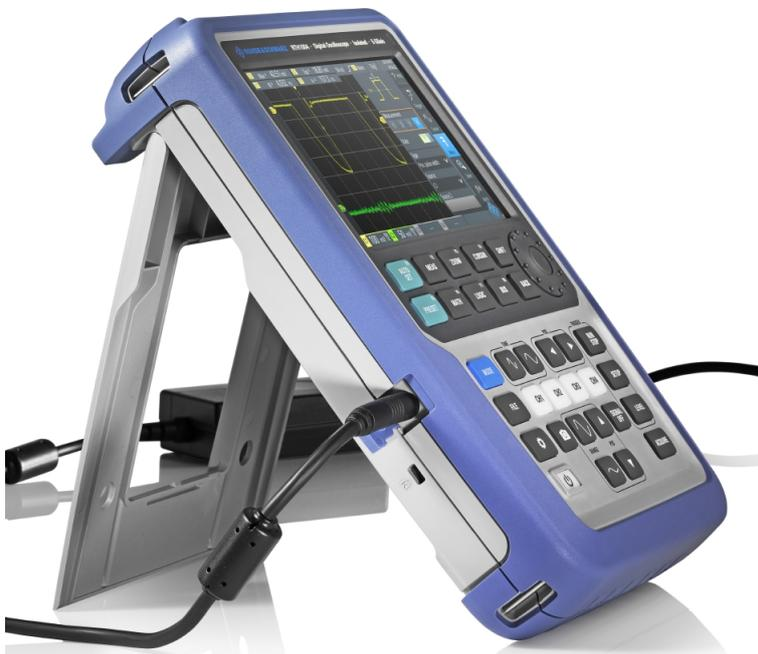
If the instrument is on, the battery status is shown on the display.
