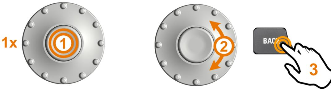
Figure 5-6: Set numerical value using the wheel
