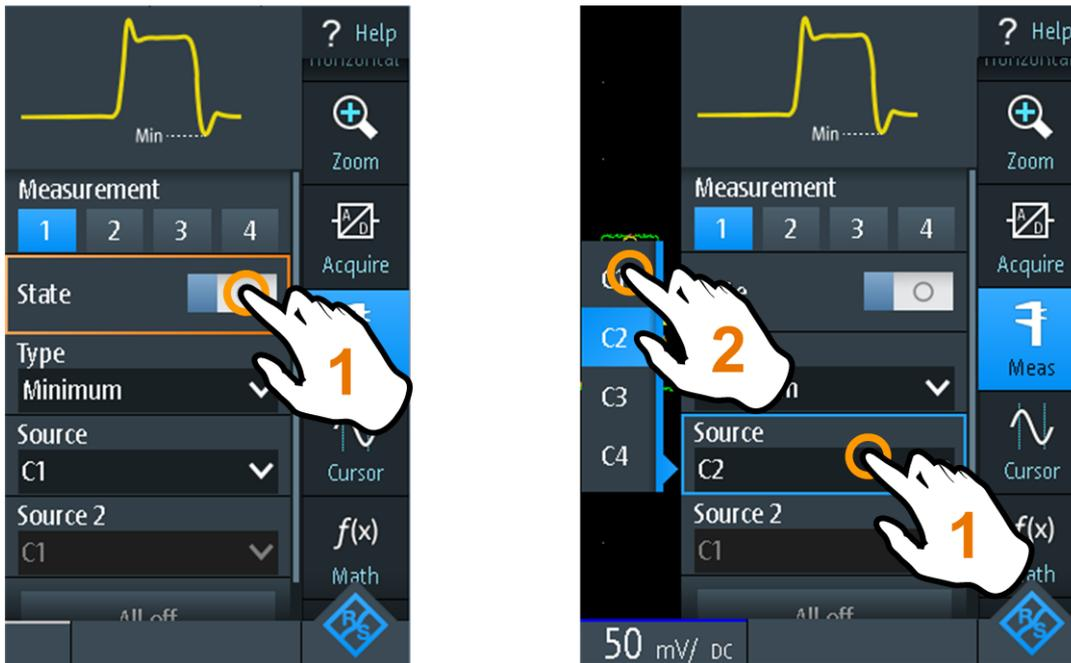
Figure 5-3: Switch on or off (left) and select a parameter value (right)
