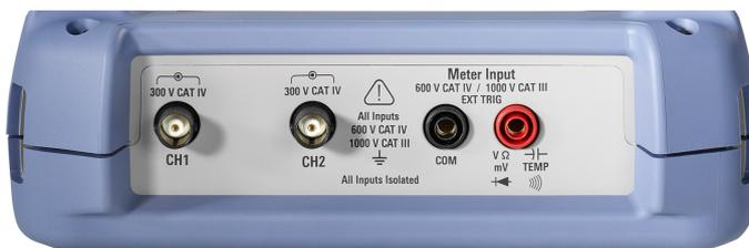
**Figure 4-3: Top view of R&S RTH1002**
