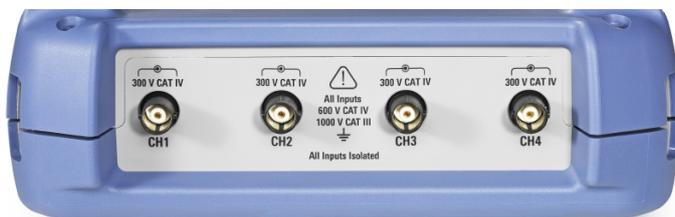
**Figure 4-4: Top view of R&S RTH1004**
