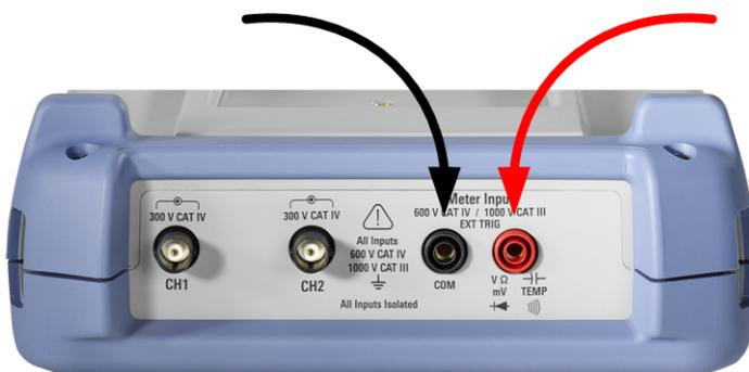
Figure 5-1: Meter inputs to connect test leads
