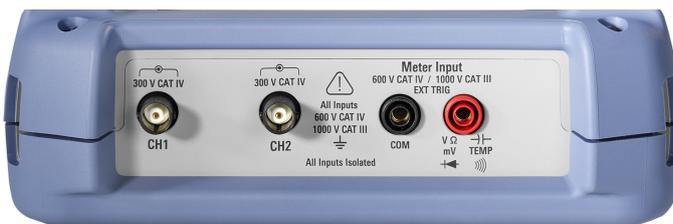
**Figure 4-3: Top view of R&S RTH1002**
