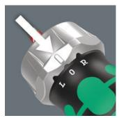
The ratchet mechanism is fine-toothed for a low return angle. The screwdriving directions right/fixed/left can be set with the reversible ring. The magnetic bit mounting is suitable for bits with 1/4" external hexagon drive as per DIN ISO 1173-C 6.3 and Wera connection series 1
