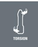
Torsion bits absorb the damaging peak torque loads in the torsion zone. This prevents premature wear and enhances the service life of the bits.
