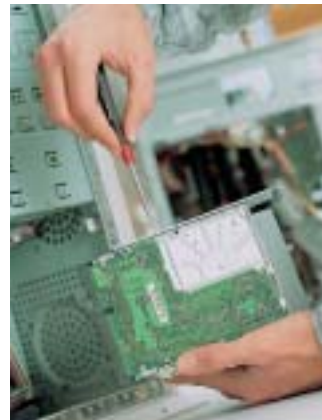
The Wiha PicoFinish features a durable chrome-vanadium-molybdenum blade.
