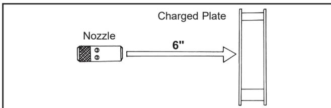
Figure 10. EOS/ESD S-3.1 decay time test set up
