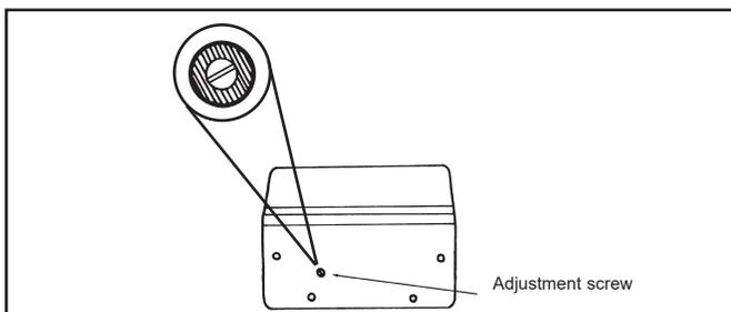
Figure 11. Balance Adjustment
