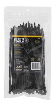
These premium, heavy duty cable ties are used to wrap and contain cables and other items. With 50 pounds of tensile strength, these ties offer a strong hold. Made of nylon for durability. Available in 7.75-Inch lengths.
