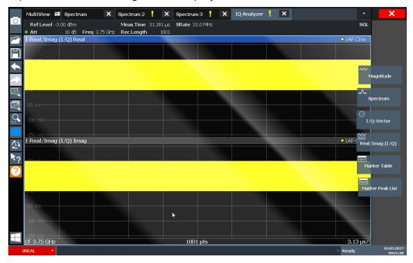
Figure 6-8: Inserting a Real/Imag diagram for I/Q analysis
