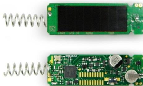
Power is provided to STM 350 by means of a small pre-installed solar cell which works in conjunction with an integrated energy storage element in order to ensure operation in periods without ambient light.
