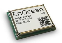
The serial interface operates according to EnOcean ESP3 standard with the option to use higher interface speeds (TURBO mode) to reduce latencies.
