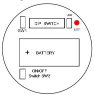
Switches 1, 2, 3 & 4 select the RF Network the IWT will transmit on. The default network for both the IWT transmitter and IWR receiver is network 1. **RF NETWORK** 1 2 3 4
