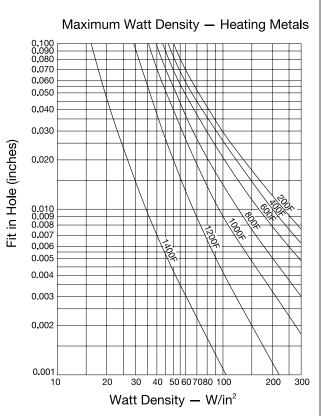
The graph shows the recommended maximum watt density for OMEGA Hi-Density cartridge heaters at different operating temperatures and fit, when the heater is installed in an oxidized mild steel block. The thermocouple is located 13 mm (½") from the heater. When heating other materials, the data needs to be extrapolated based on the thermal conductivity of the material. Consult OMEGA with your requirements.
