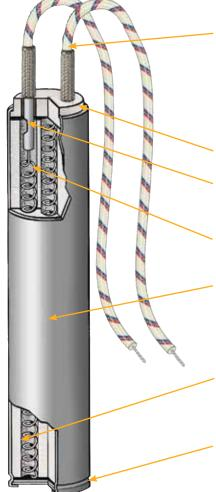
The standard termination for low-density cartridge heaters is Type F, consisting of 254 mm (10") internally connected flexible lead wires with high temperature insulation, UL approved for 300 or 600V service and temperature rated to 250°C (482°F). **Note:** To meet the requirements of your application we offer over 40 standard termination styles to select from that will solve many of the most common application problems.
