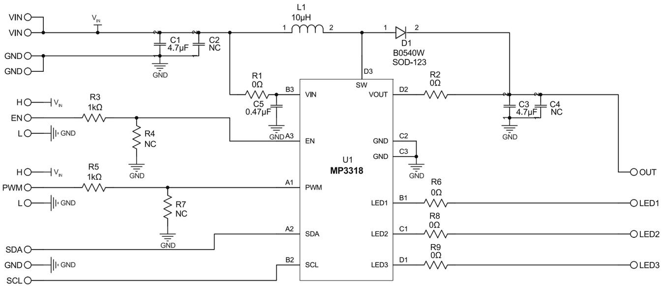
Figure 2: Typical Application Schematic with 3 strings (7 LEDs/string, 20mA/String)
