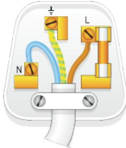
After unpacking your amplifier check that it is factory fitted with a three pin 'grounded' (or earthed) plug. Before plugging into the power supply ensure you are connecting to a grounded earth outlet.
