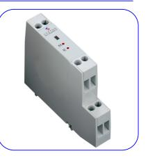
The SEM213/P is a cost effective "smart" DIN rail mount transmitter that accepts resistance temperature sensors and converts sensor output over a configured range to a standard industrial (4 to 20) mA transmission signal.
