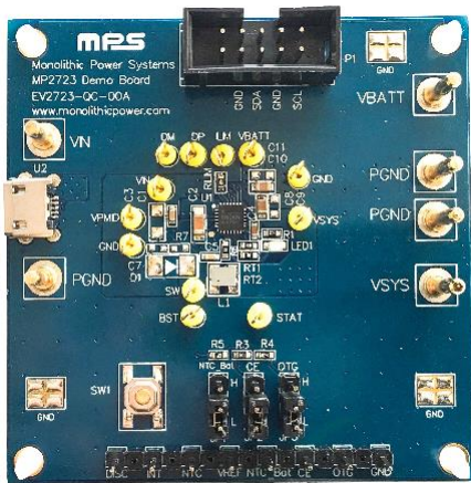
Figure 2: EV2723-QC-00A Evaluation Board
