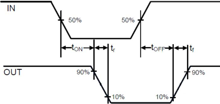
**Figure 1.** Switching Time Waveform Definitions
