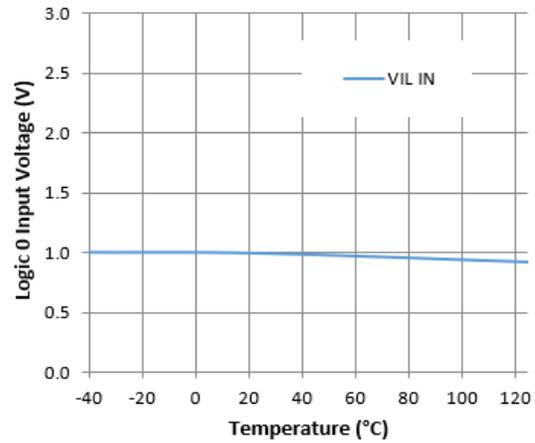
**Figure 19.** Logic 0 Input Voltage vs. Temperature
