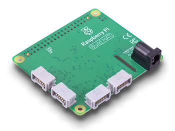
The Raspberry Pi Build HAT is an add-on board designed in collaboration with LEGO® Education to make it easy to control LEGO® Technic™ motors and sensors with Raspberry Pi computers.
