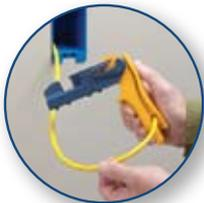
1. Strip cable jacket with a standard cable stripper or the built-in cable stripper.
