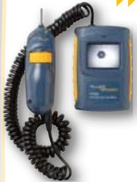
The FiberInspector Mini video microscope enables inspection of end-faces on all types of installed fiber. The portable video microscope projects a crisp, clear image of microscopic debris and end-face damage.
