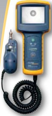
The FiberInspector Pro is a portable, dual magnification video microscope which enables inspection of all types of installed fiber terminations in hardware devices and patch panels. The video microscope projects a crisp, clear image of microscopic debris and end-face damage.
