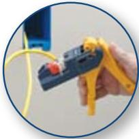
4. Ensure jack is completely and securely inserted in jack holder bed with IDC slots facing the blades.
