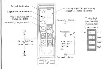
The output timing logic function (on sensor models with T9 model **number suffix**) is selected at the timing logic programming switches, according to the table (right). The output timing logic delays are set at the single-turn time adjustment potentiometer. When the timing function involves more than one time (as in ON and OFF delay, ON-delayed one-shot, and ON-delayed limit timer functions), the potentiometer sets both times to the same value.
