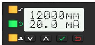
Figure 2. Display shown in Run Mode
