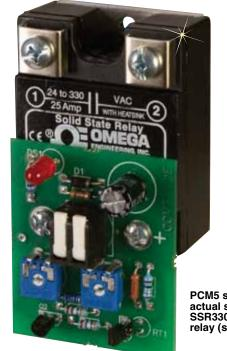
PCM5 shown actual size, mounted on SSR330DC25, solid state relay (sold separately).
