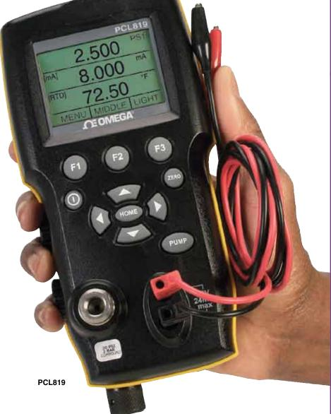
can generate vacuum or pressure from -12 to 300 psig.
