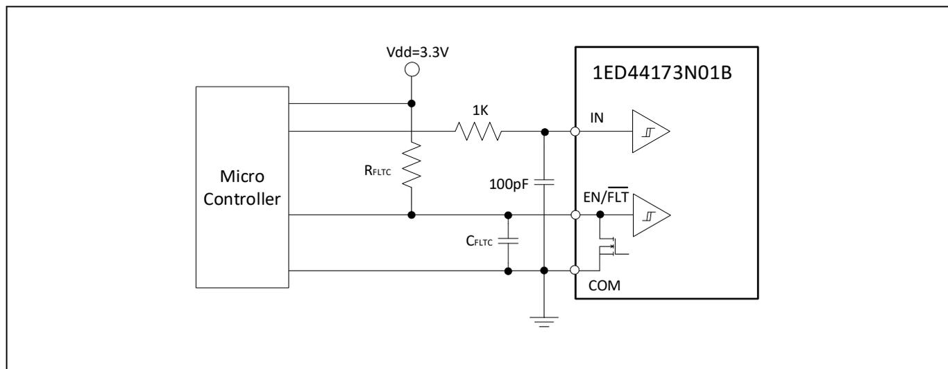
**Figure 3 Recommended microcontroller I/O interface circuit**
