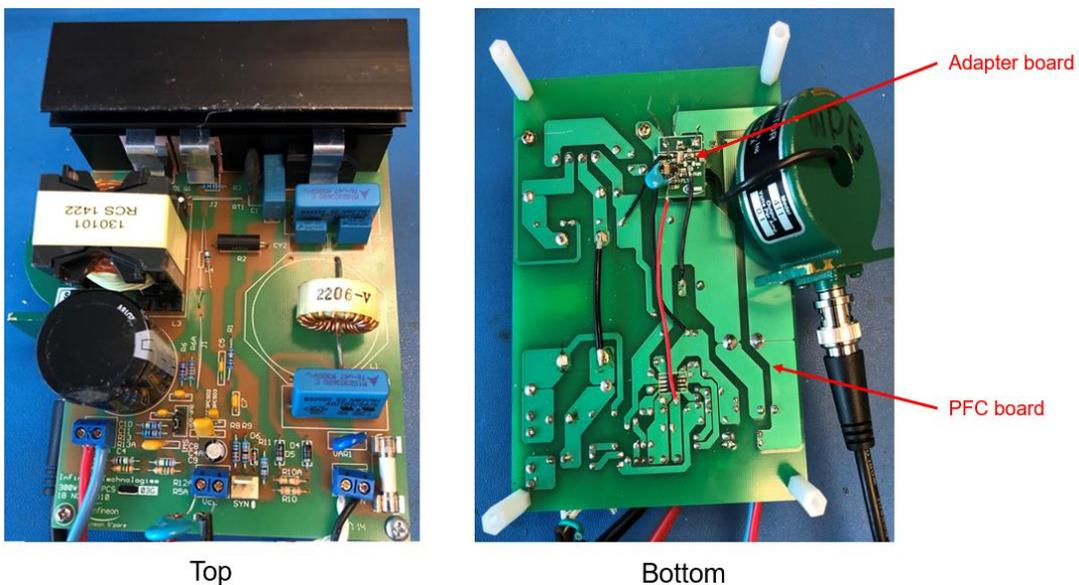
Figure 16 Connection between PFC board and adapter board
