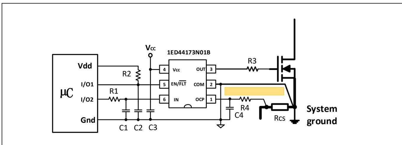
Figure 6 Recommended layout pattern for OCP & SCP function
