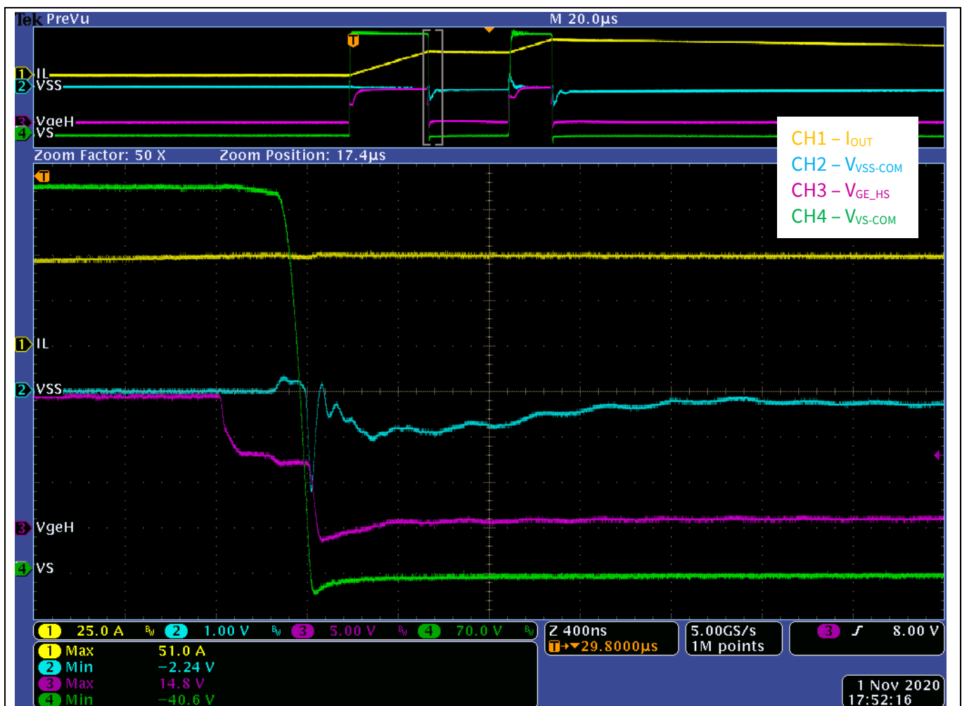
Figure 28 Negative V_s and V_{SS} transient at 50 A switching current
