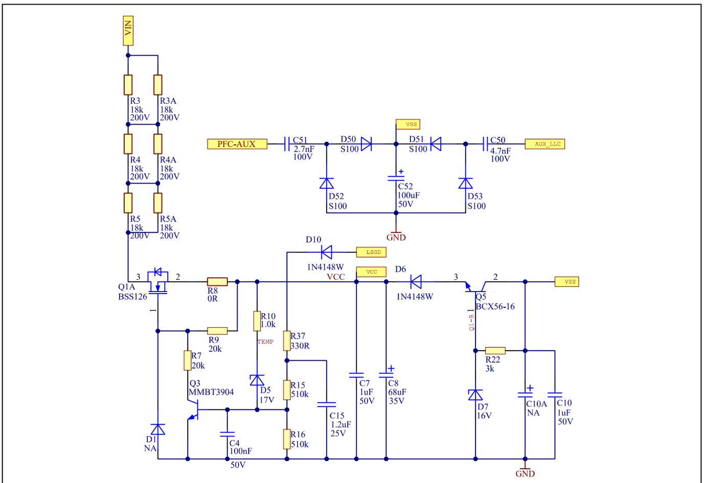
**Figure 4** Schematic of the start-up and V<sub>CC</sub> circuit
