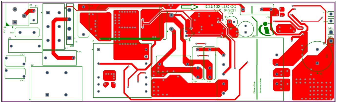
Figure 7 Layout of the through-hole component side
