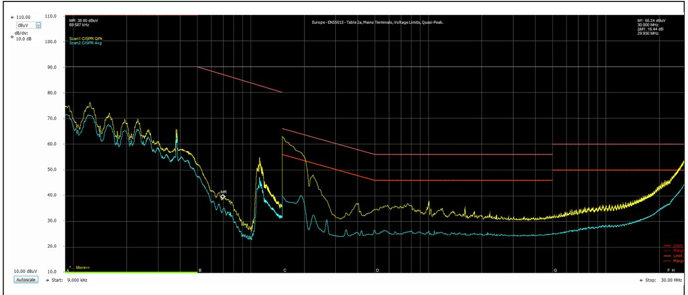
**Figure 26 Conducted EMI at 230 V<sub>RMS</sub> input and 130 W output**
