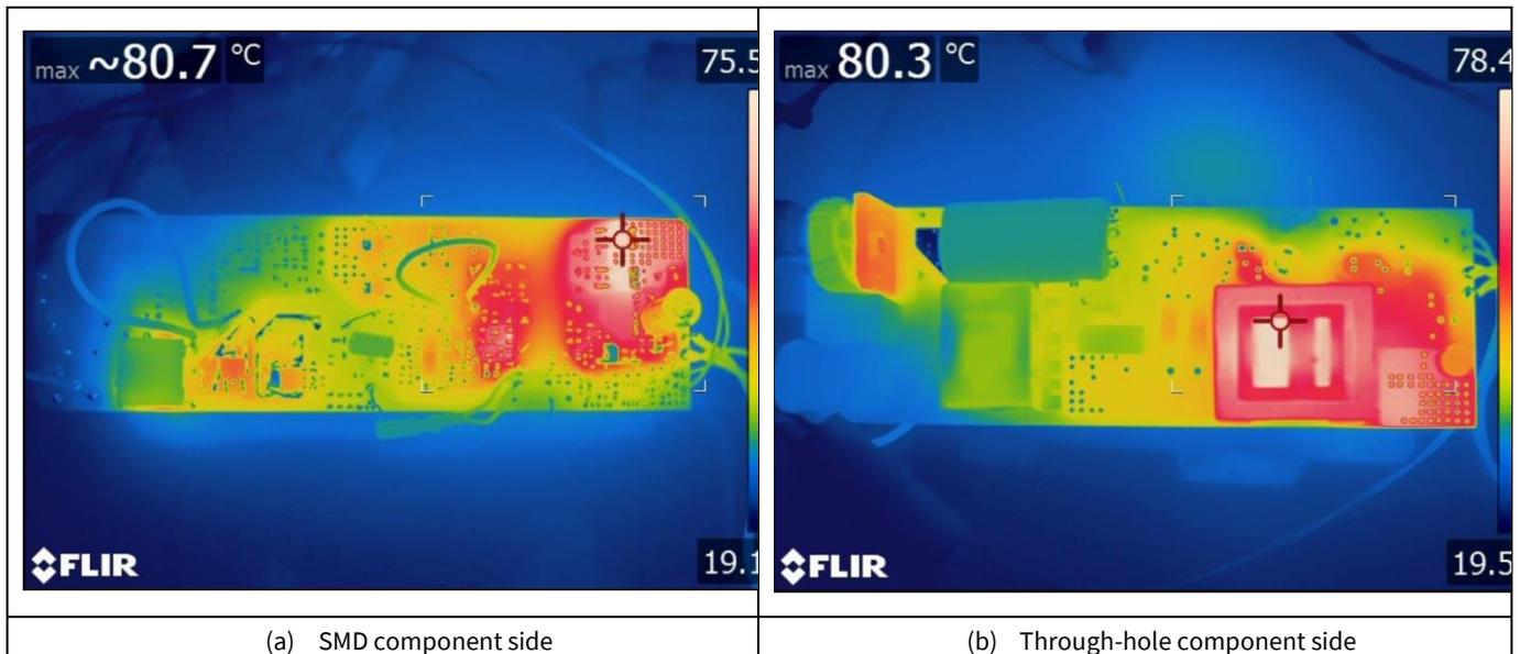
**Figure 25** Infrared images at 230 V<sub>RMS</sub>, 76 V<sub>LED</sub> and 130 W
