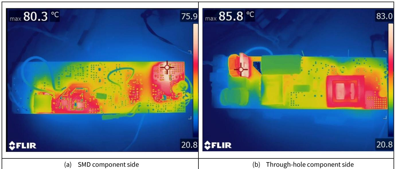
**Figure 24** Infrared images at 120 V<sub>RMS</sub>, 76 V LED and 130 W
