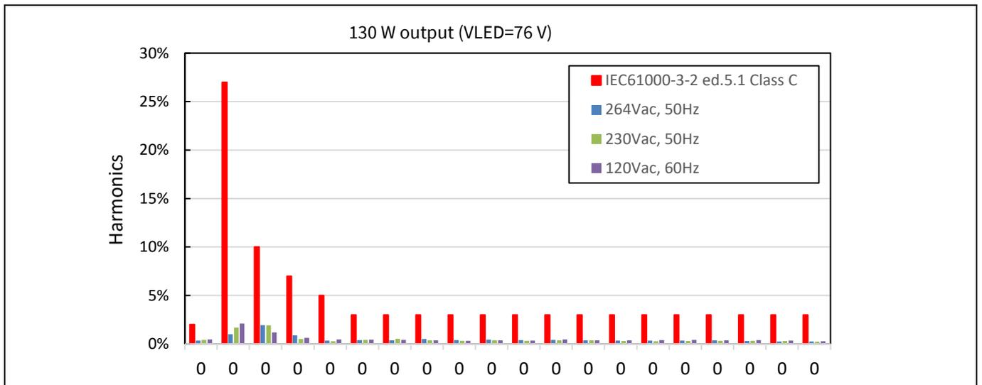
Figure 14 Input current harmonics at 130 W load
