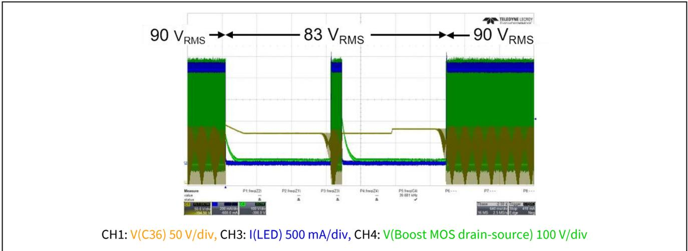
**Figure 22** Brown-out protection (brown-out point at 83 V<sub>RMS</sub>)
