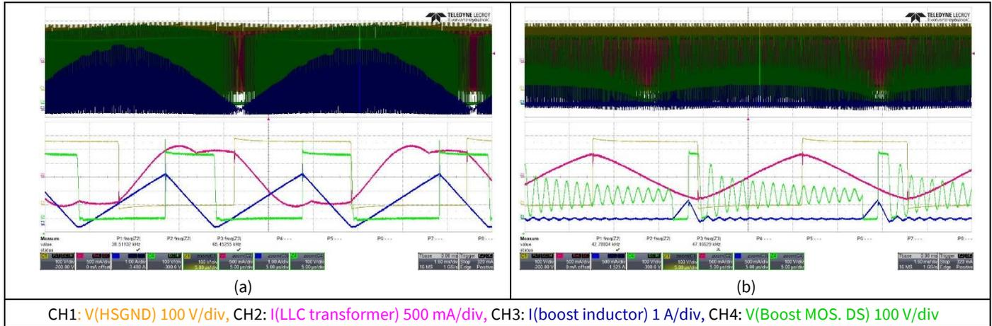
**Figure 18** Boost and LLC waveforms at 120 V<sub>RMS</sub> (a) V<sub>dim</sub> = 10 V, V<sub>LED</sub> = 76 V and (b) V<sub>dim</sub> = 0.1 V, V<sub>LED</sub> = 65 V
