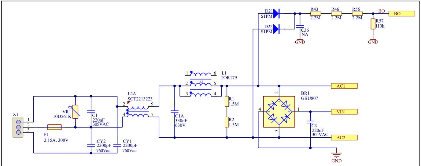
**Figure 3** Schematic of the input EMI filter and the brown-out sensing network
