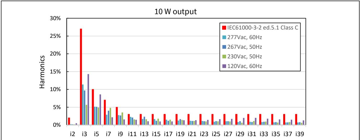
**Figure 15** Input current harmonics at 10 W load
