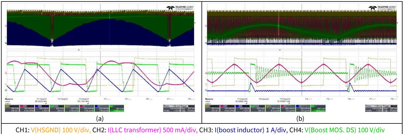
**Figure 16** Boost and LLC waveforms at 230 V<sub>RMS</sub> (a) V<sub>dim</sub> = 10 V, V<sub>LED</sub> = 76 V and (b) V<sub>dim</sub> = 0.1 V, V<sub>LED</sub> = 65 V
