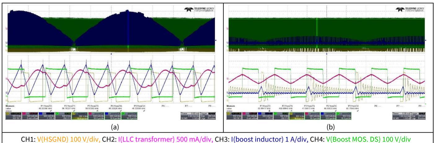
**Figure 19** Boost and LLC waveforms at 120 V<sub>RMS</sub> (a) V<sub>dim</sub> = 10 V, V<sub>LED</sub> = 46 V and (b) V<sub>dim</sub> = 0.1 V, V<sub>LED</sub> = 39 V
