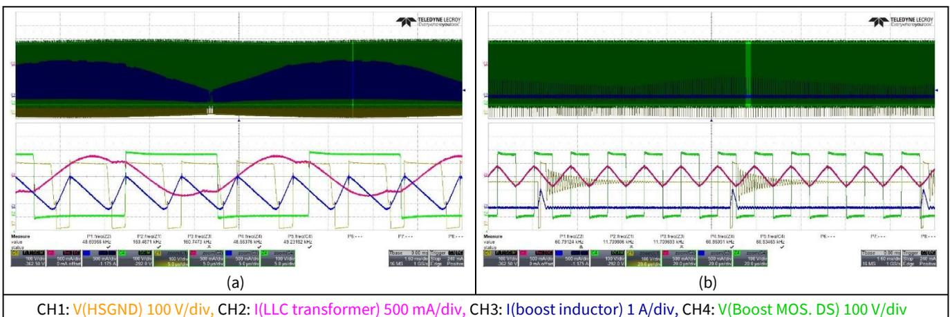
**Figure 17** Boost and LLC waveforms at 230 V<sub>RMS</sub> (a) V<sub>dim</sub> = 10 V, V<sub>LED</sub> = 46 V and (b) V<sub>dim</sub> = 0.1 V, V<sub>LED</sub> = 39 V
