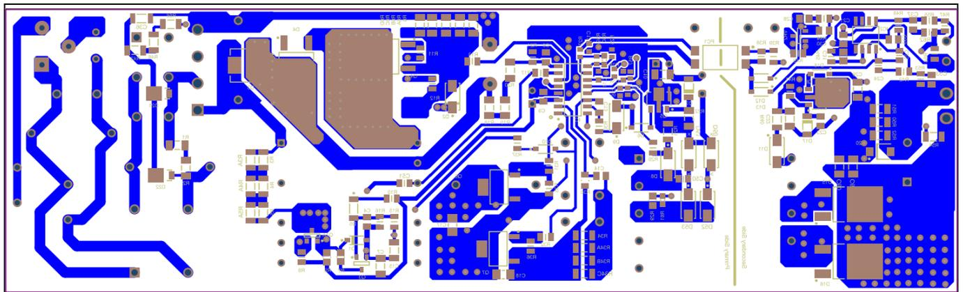
Figure 8 Layout of the SMD component side
