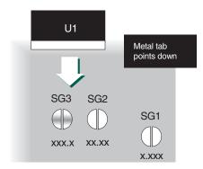
Figure 2. Installing U1
