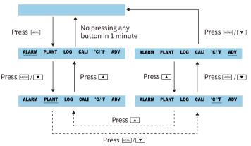
To select the function, press when it is underlined by the flashing bar. Note that after 30 seconds if nothing is pressed, the Main Menu will disappear and the device will revert to the normal state.
