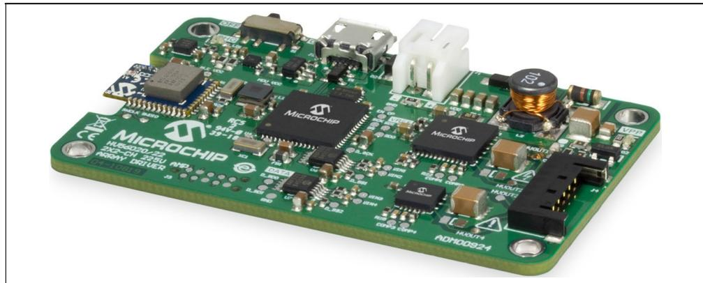
**FIGURE 1-3:** HV56020/22 Evaluation Board Side View.
