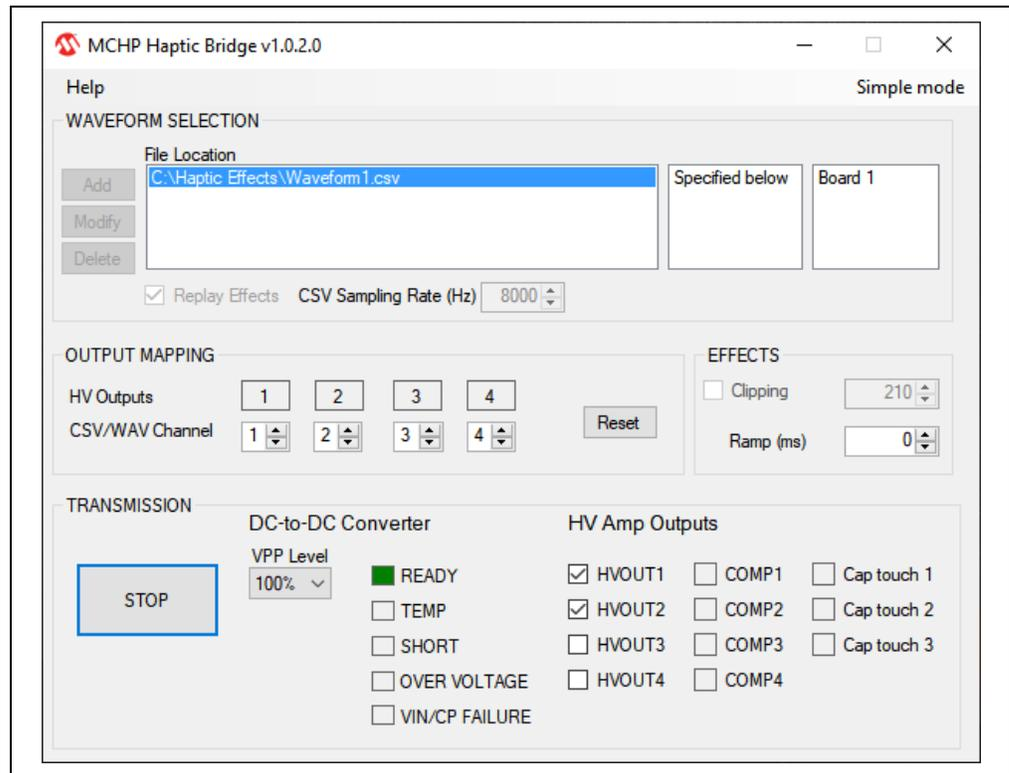
**FIGURE 2-19:** Successful Transmission.
