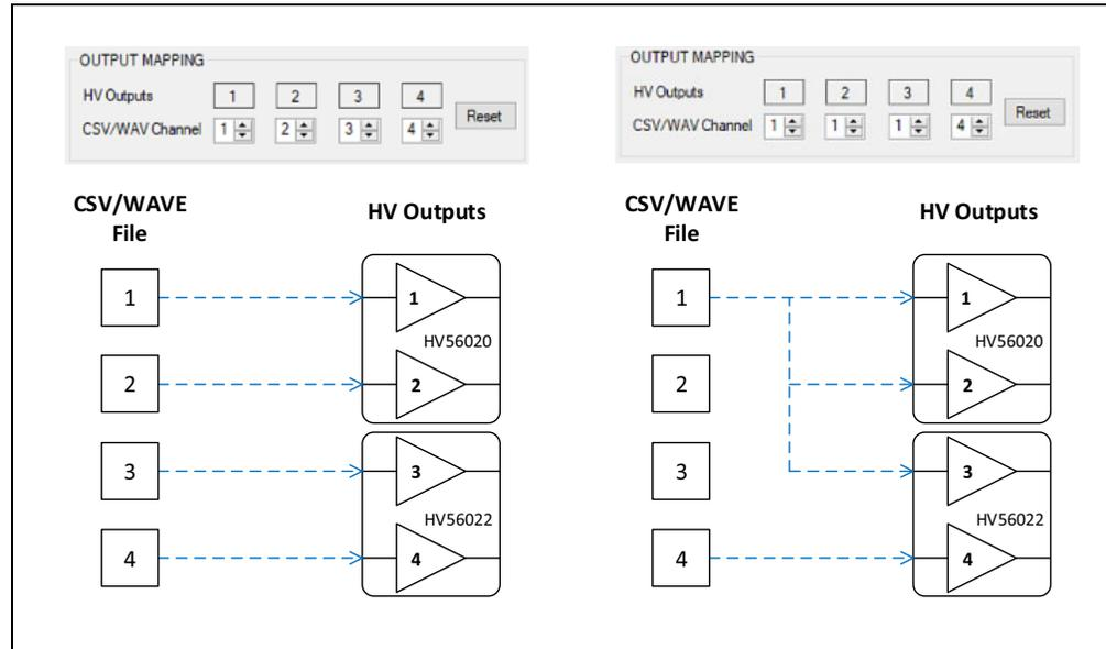
**FIGURE 2-15:** Channel Mapping.
