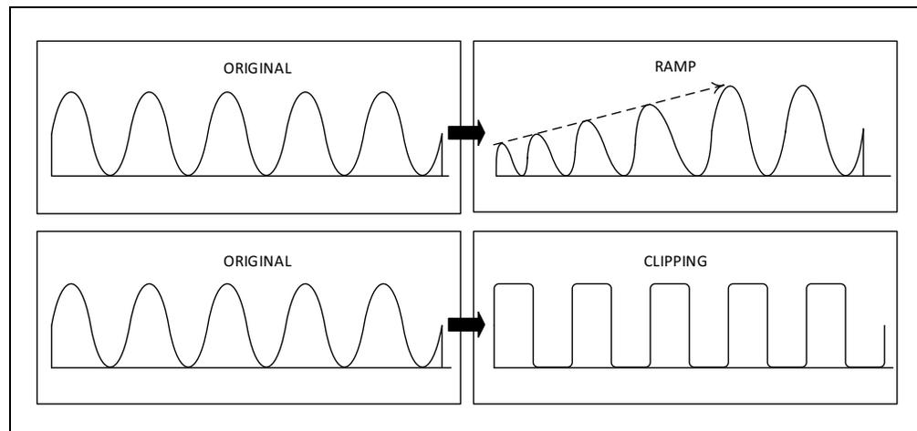
**FIGURE 2-16:** Clipping and Ramp Effects.
