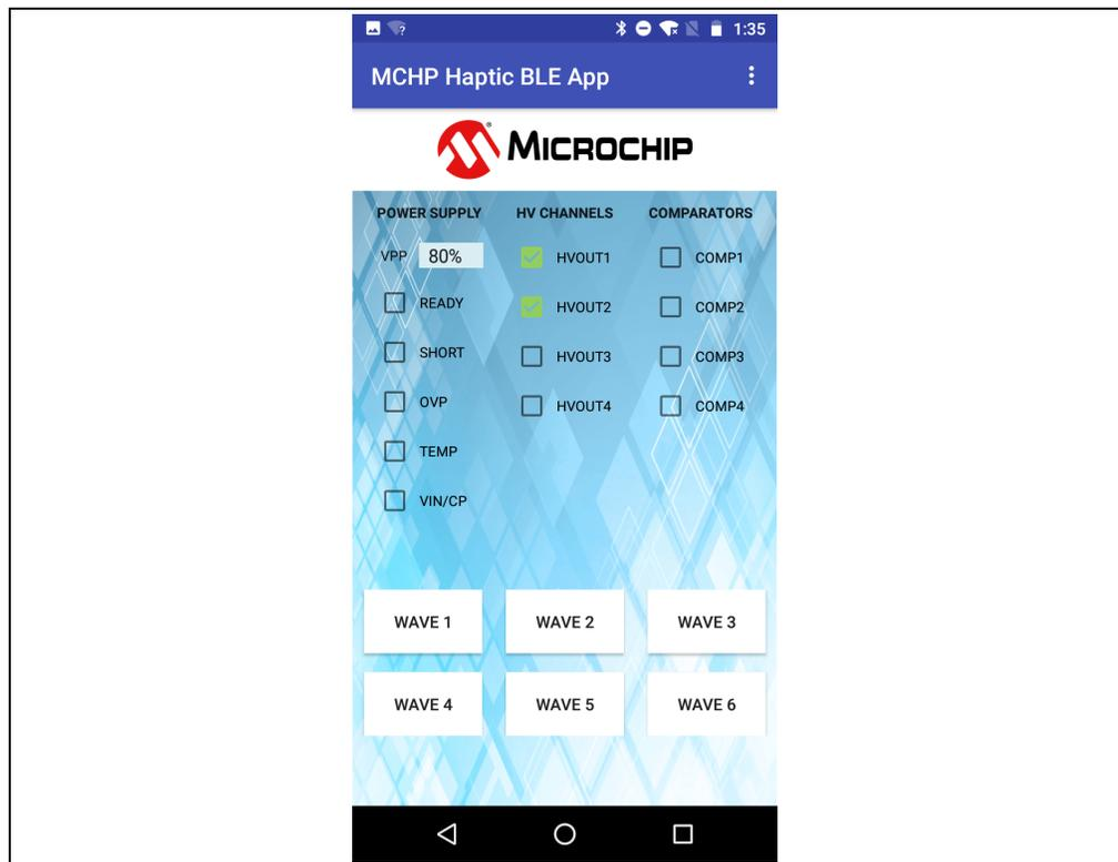
**FIGURE 2-22:** *HV CHANNELS Selection.*
