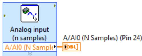
Figure 9. Analog Input Using an Express VI
