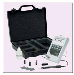
Kit includes dissolved oxygen meter and probe, 2 replacement membranes, electrolytic filling solution, stirrer bar and guard shield assembly, battery and complete operator's manual.
