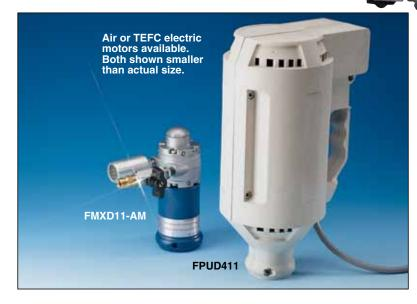
The air-driven ¾ HP motor operates with 10 to 15 CFM air at 3.4 to 6.2 bar (50 to 90 psig), and includes a flow regulator and muffler.
