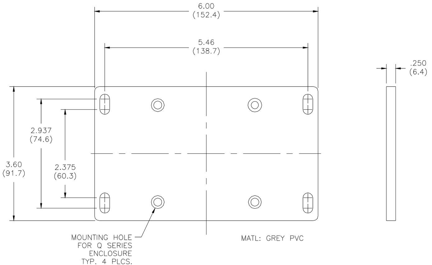
**Figure 2-3 Wall or Pipe mount Bracket**
