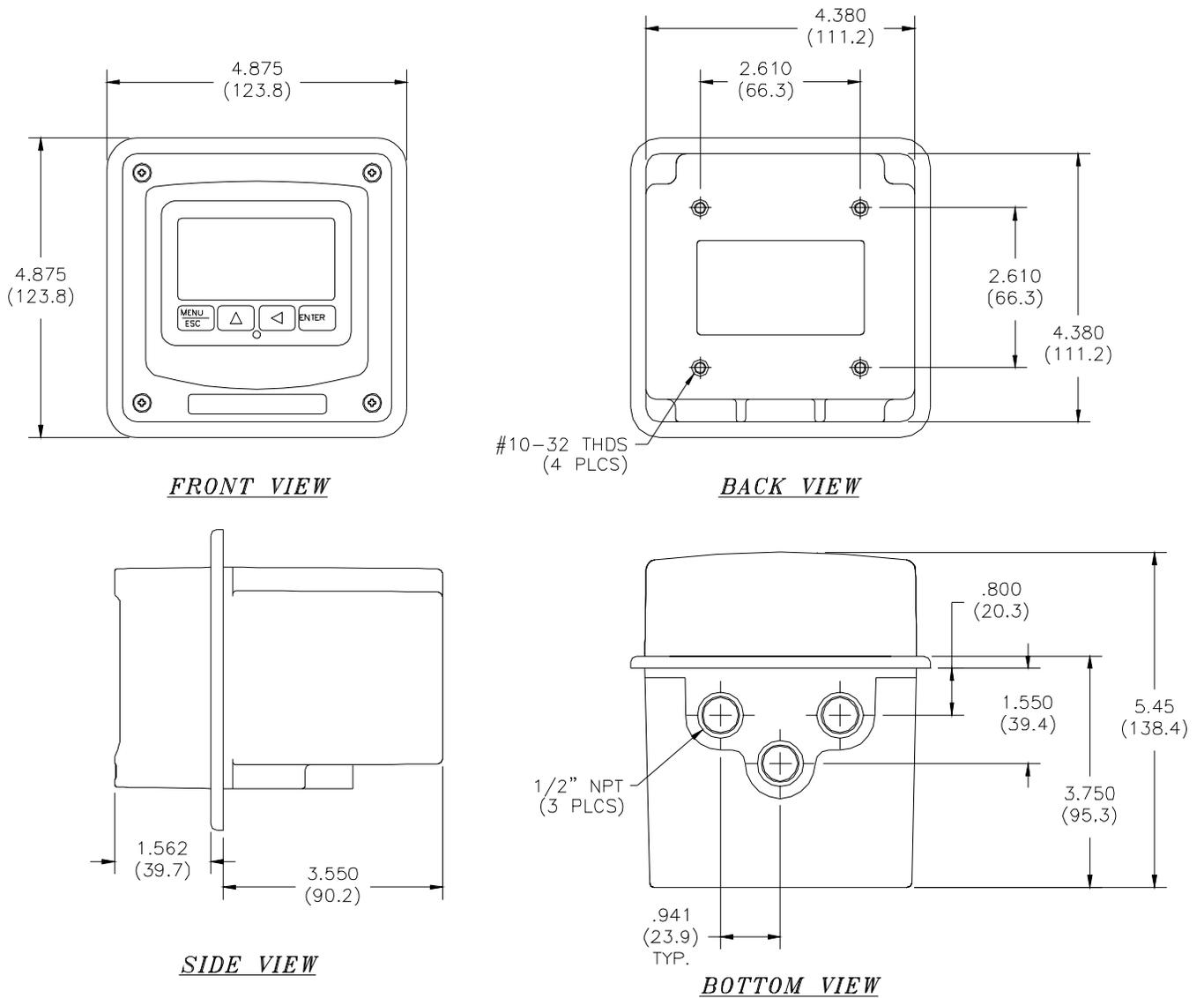
**Figure 2-1 Enclosure Dimensions, AC Powered Units**
