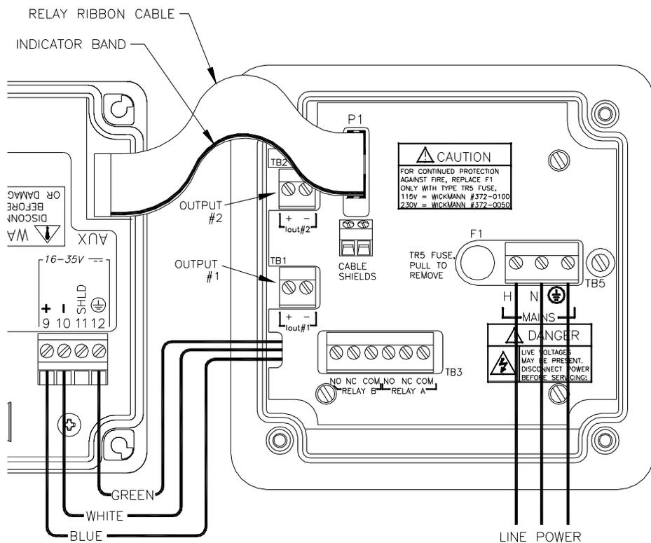
**Figure 4-3 Line Power Connection**
