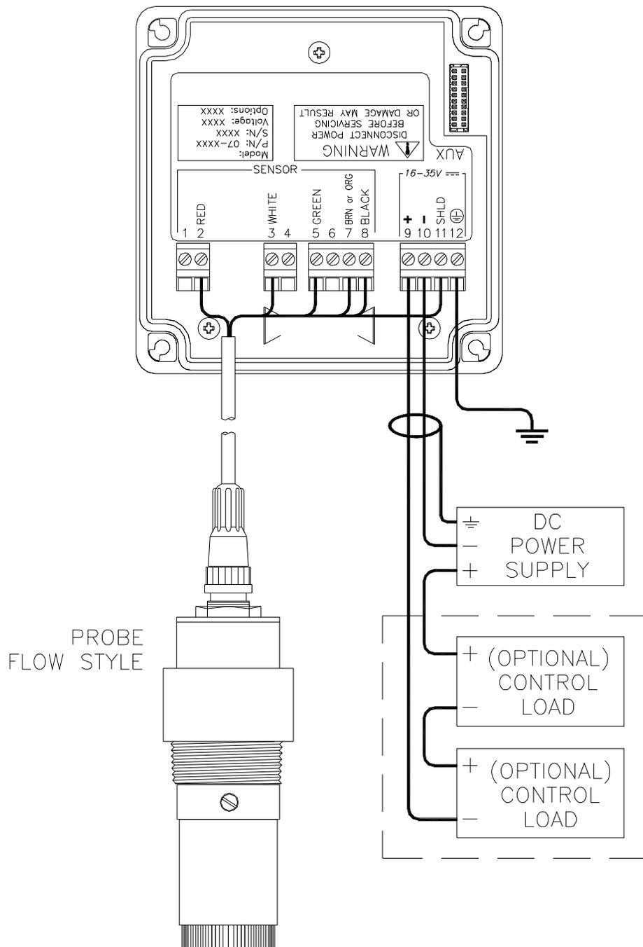
**Figure 4-1 Loop-Power Connection**
