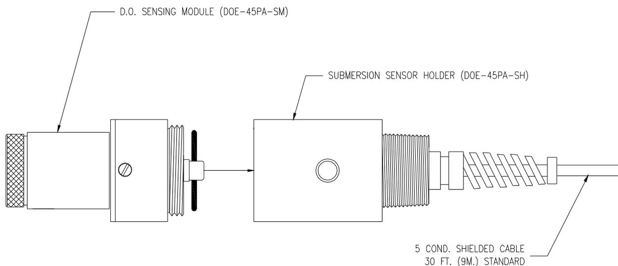
**Figure 5-1 Submersible Oxygen Sensor Assembly**
