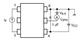
Fig. 13.1.1 I<sub>OPH</sub> Test Circuit
