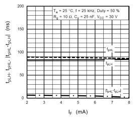
Fig. 13.2.12  $\,$   $\,$   $t_{pLH},\,t_{pHL},\,|t_{pHL}$  -  $t_{pLH}|$  -  $I_{F}$
