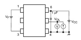
Fig. 13.1.4 V<sub>OL</sub> Test Circuit
