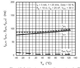
Fig. 13.2.11  $t_{pLH}$ ,  $t_{pHL}$ ,  $|t_{pHL} - t_{pLH}| - T_a$
