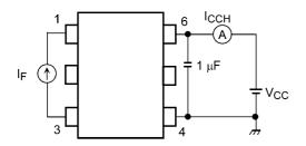
Fig. 13.1.5 I<sub>CCH</sub> Test Circuit
