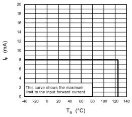
Fig. 13.2.2 I<sub>F</sub> - T<sub>a</sub>
