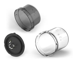
THE BASE ASSEMBLY INCLUDES POWER TWIST LOCK TERMINALS, SPRING LEAF SIGNAL TERMINALS, AND AN INTEGRAL SEALING GASKET. COUPLE THAT WITH AN IK08 RATED COVER AND THE ASSEMBLED NETWORK LIGHTING CONTROL ACHIEVES AN IP66 SEAL RATING.
