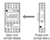
The functions of the Main Unit and Probe Unit are shown in the figure on the right. The Main Unit correspond to a Megohmmeter, and the Probe Unit correspond to a measurement probe with internal contacts. The Main Unit turns ON these contacts in sequence and measure multiple loads individually. Up to eight Probe Units can be connected to one Main Unit.
