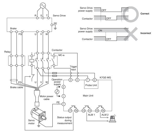
The figure shows a simplified view of the wiring for status output during measurement, and ALM 1 and ALM 2 outputs. Use an appropriate relay for relaying in consideration of the switching capacity of the output transistor. The specifications of the output transistor for the K7GE-MG are 24 VDC (+10%), 50 mA max.
