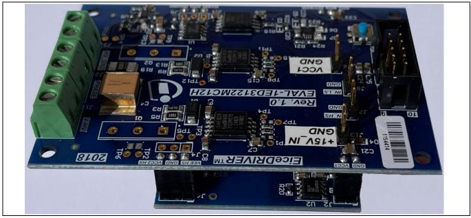
Figure 5 View of complete solution (power supply board + isolated gate driver eval-board)
