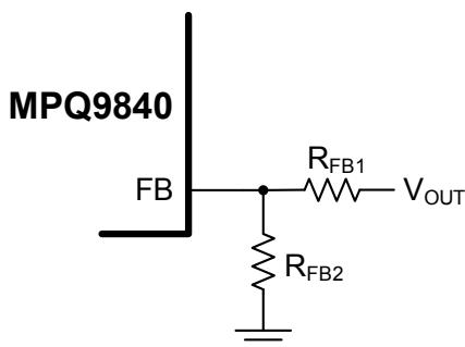
**Figure 1: Feedback Circuit**
