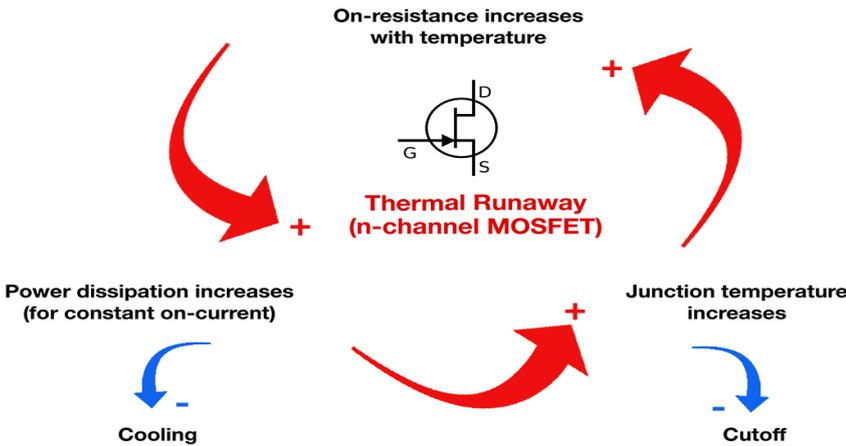
Cause diagram for thermal runaway at an n-channel MOSFET
