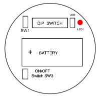
Switches 1, 2, 3 & 4 select the RF Network the IWTT will transmit on. The default network for both the IWTT transmitter and IWR receiver is network 1.
