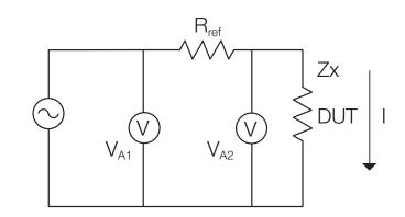
Figure 2. The I-V method test circuit.
