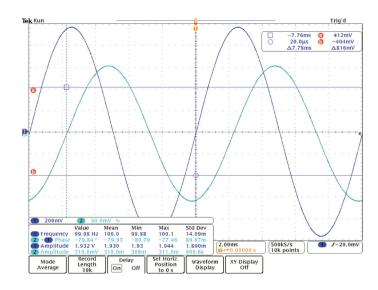
Figure 4. Voltage waveforms and measurements taken at nodes A1 and A2.
