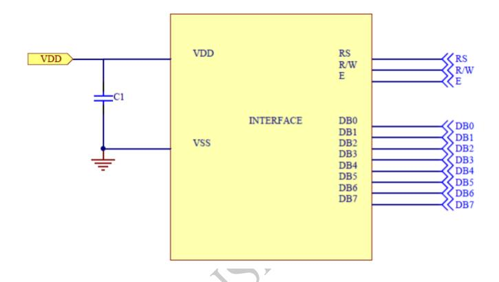
Pin connected to MCU interface: RS, R/W, E, DB0~DB7
