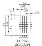
The non-specified tolerance of dimension is  $\pm 0.3$  mm .
