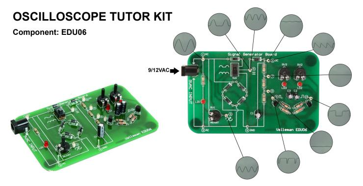
Learn how to get the most out of your digital oscilloscope. The board generates a number of safe 'real-world' signals, which we will use to perform measurements. Get familiarized with AC, DC and frequency measurements, sine and square waves, power supply ripple, full and half wave rectifiers, oscillators etc...
