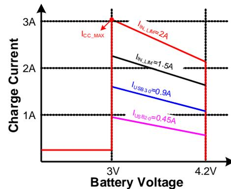
**Figure 7:  $I_{CHG}$  Variation with Different Input Current Limit**
