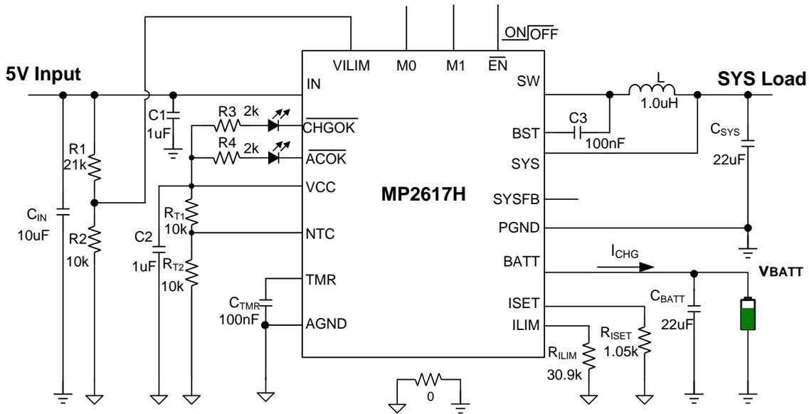
**Figure 9: Typical Charge Application Circuit for 5V input**
