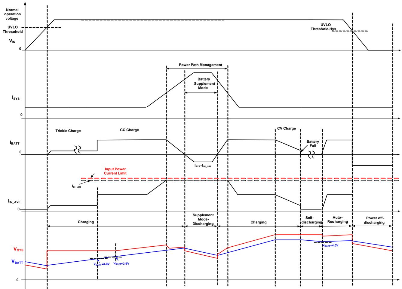
**Figure 6: MP2617H Operation Process under No Fault Condition**
