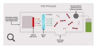
The PAS principle works as follows. Pulses of light from an infrared source pass through an optical filter tuned specifically to the  $CO_2$  absorption wavelength ( $\lambda$ = 4.2  $\mu$ m). The  $CO_2$  molecules inside the measurement chamber absorb the filtered light, causing the molecules to shake and generate a pressure wave with each pulse. This is called the photoacoustic effect. The highly sensitive MEMS
