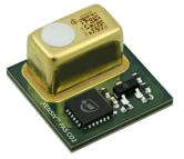
The XENSIV™ PAS CO2 integrates on the PCB the photoacoustic (PAS) transducer, including a detector, infrared source and optical filter; a microcontroller for signal processing and algorithms; and a MOSFET chip to drive the infrared source. The integrated microcontroller runs ppm calculations as well as advanced compensation and configuration algorithms.
